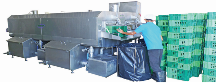
DUAL-LANE WITH 4 WASHING ZONE + BLOW OFF
