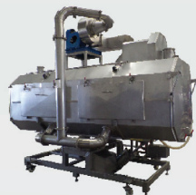
Drum Dryer (Heater)
