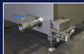
DRAIN DOOR & DRAIN VALVE
