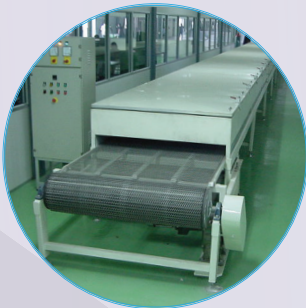
INFARED HEATER TUNNEL OVEN
