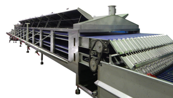
Steam tunnel Cooker
